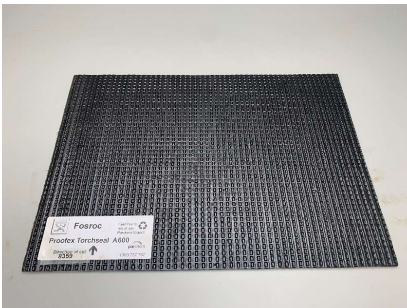
FIGURE 1 TOP FACE OF PROOFEX TORCHSEAL A600
