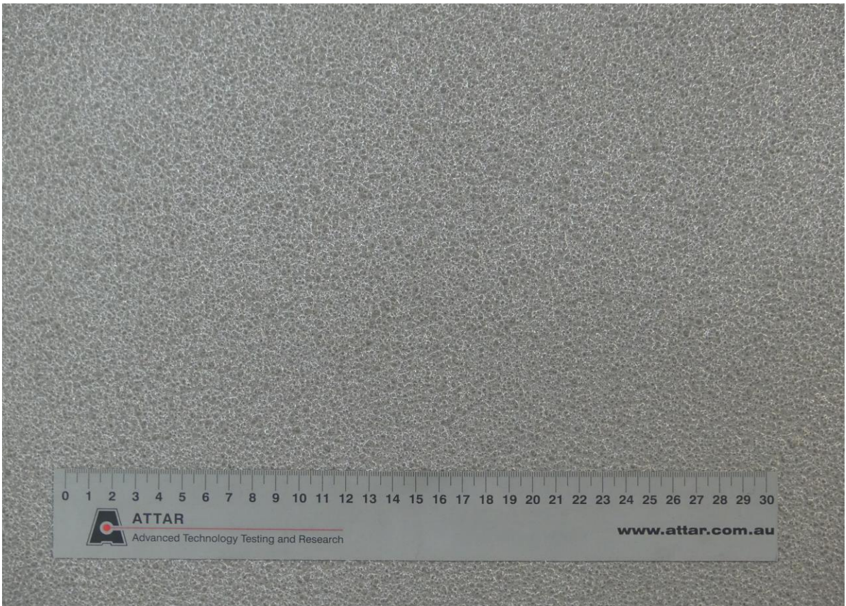
Figure 1: Fosroc Nitoflor FC150 HP-FC + Fosroc Nitoflor Anti-Slip Grains 01 Silica Sand 16/30# + Fosroc Nitoflor FC150 HP-FC
