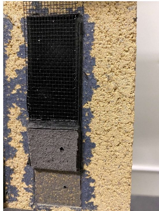
FIGURE 4 IMAGES OF TEST SAMPLE PERFORMING ADHESION-IN-PEEL
